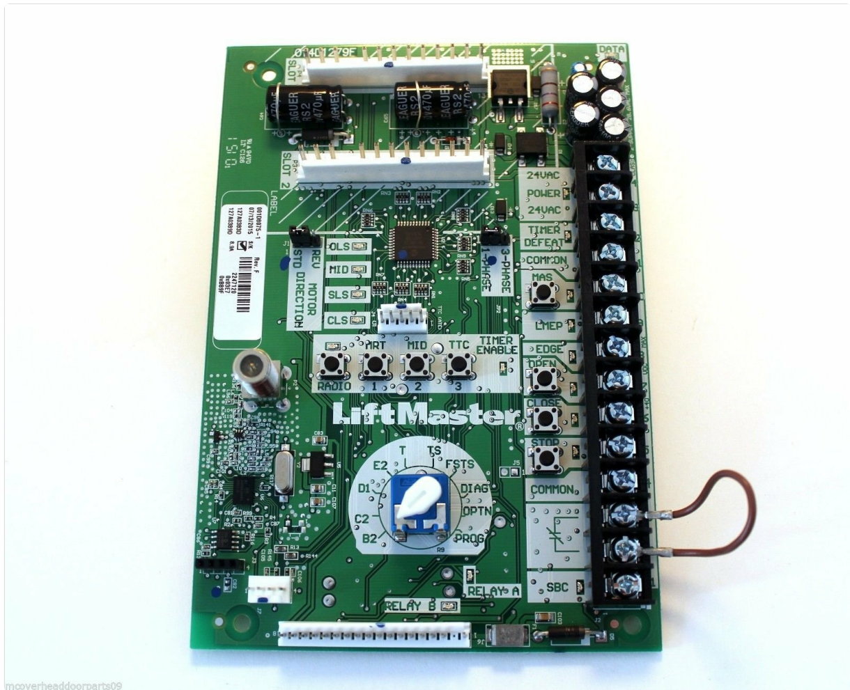
Image of the LiftMaster L5 Logic Control Board, showing its electronic components and connectors.
