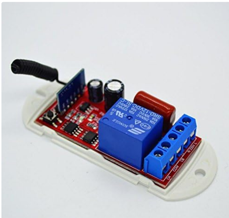
Figure 1: Internal view of the wireless smart switch module. This image displays the red circuit board, the blue relay, capacitors, and the
