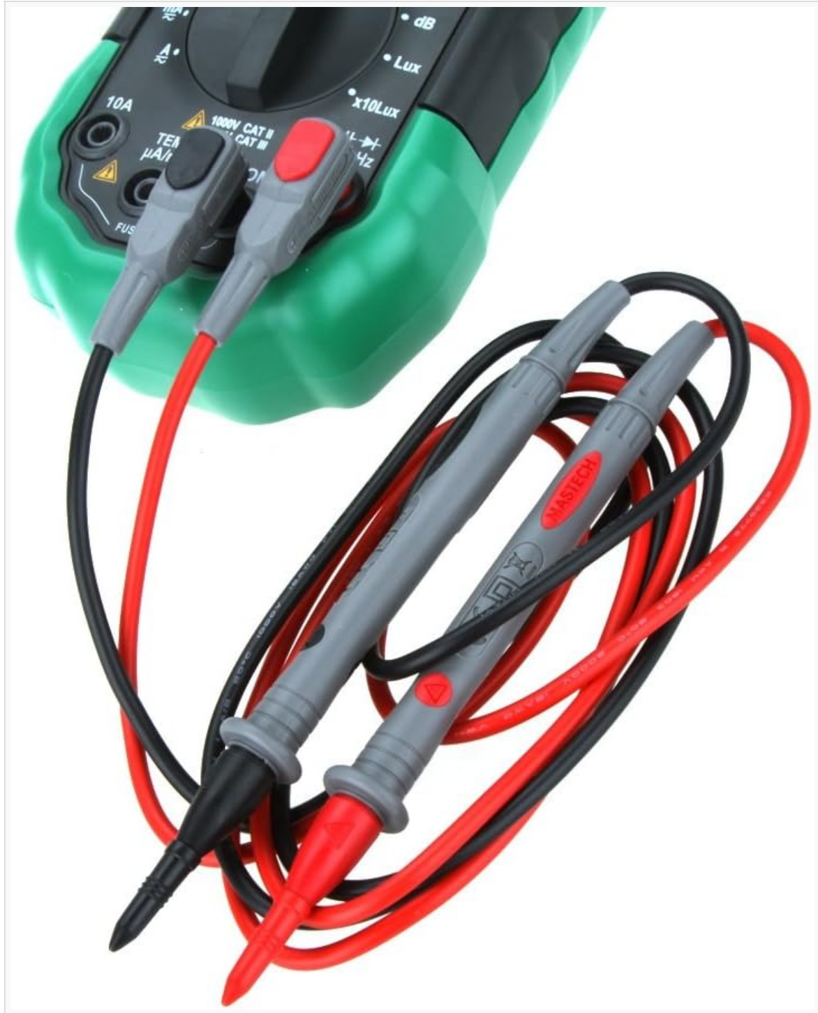
Figure 5.2: The MS8229 Multimeter with red and black test leads properly inserted into the input jacks.
