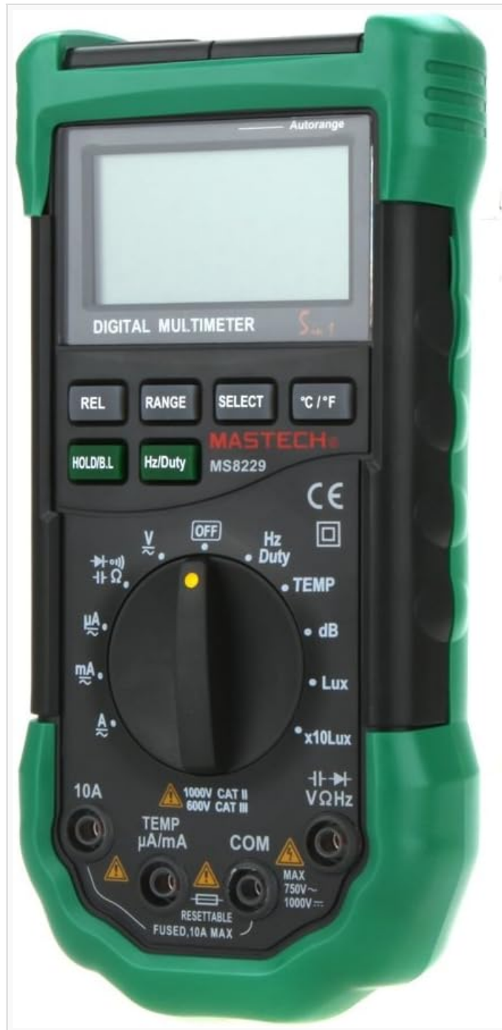
Figure 1.1: Front view of the MS8229 Digital Multimeter, showing the display, rotary switch, and input jacks.
