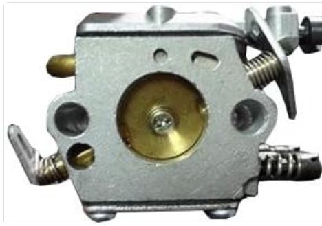
Figure 4.3: Side view of the carburetor, showing the fuel inlet connection.
