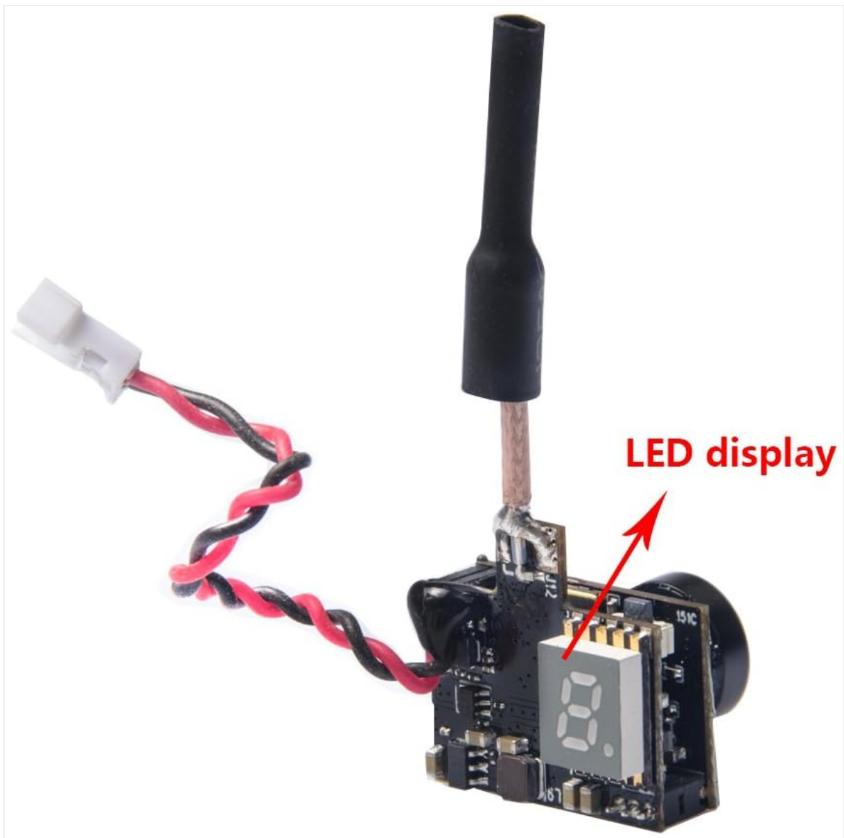
Figure 2.3: Close-up view of the AKK BA3's LED display, which indicates current settings.
