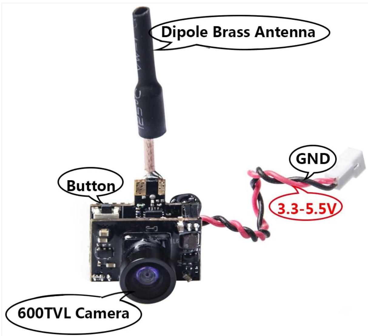
Figure 2.2: Labeled components of the AKK BA3 unit, including the button, power input, antenna, and camera lens.
