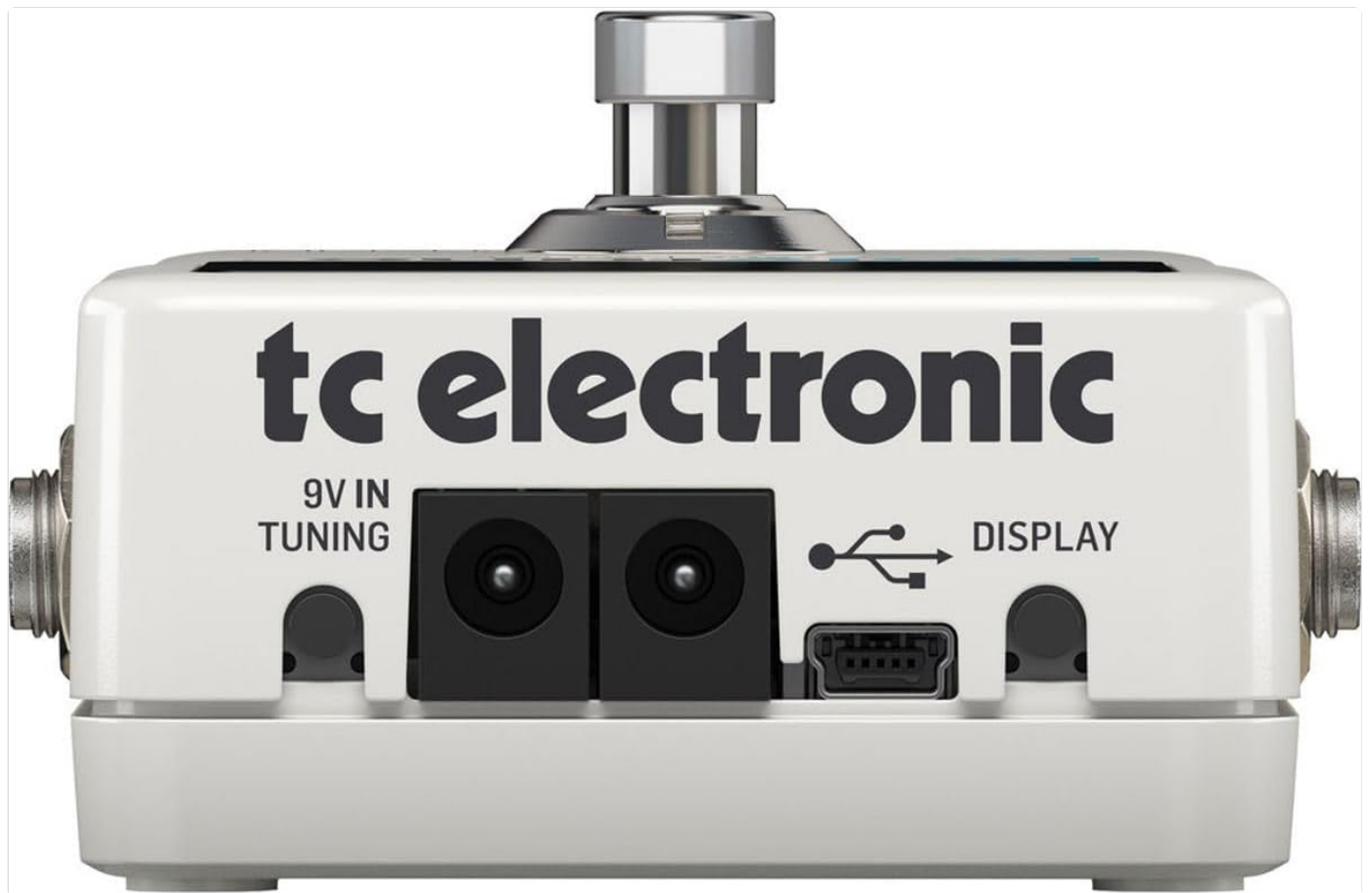
Figure 2: Rear view of the POLYTUNE 3, highlighting the input, output, and 9V power connections.
