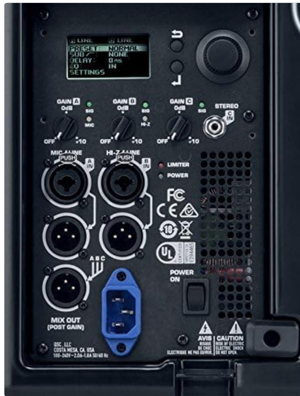
Figure 3.3: Detailed view of the K10.2's rear panel, showing input options and control knobs.
