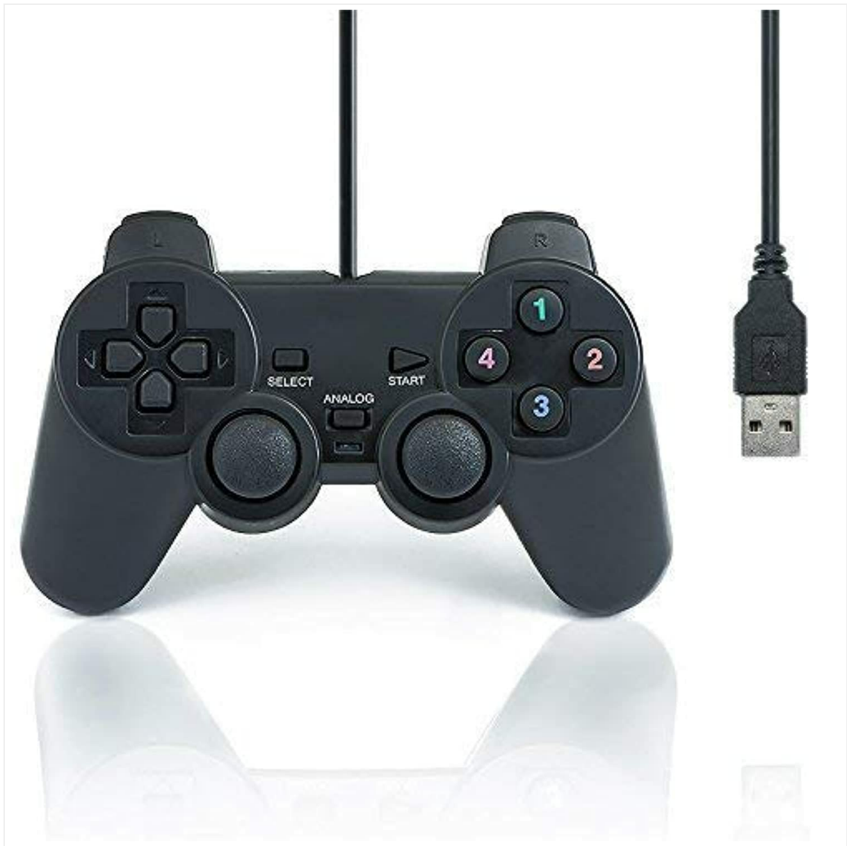
Image: Front view of the QUMOX Wired USB Gamepad, showing the dual analog sticks, D-pad, action buttons (numbered 1-4), and central Select, Analog, and Start buttons.
