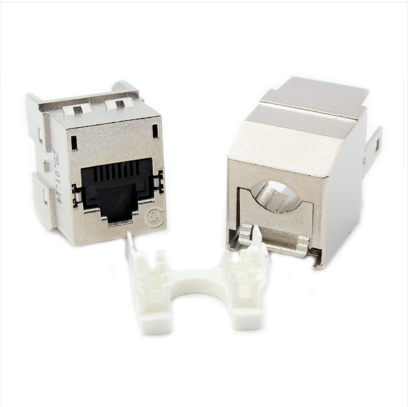
Figure 3: Molex KSJ-00062-04 jack with wire cap and internal module separated. This view demonstrates how the jack module fits into the metal housing and how the white plastic wire cap secures the terminated wires, ready for final assembly.
