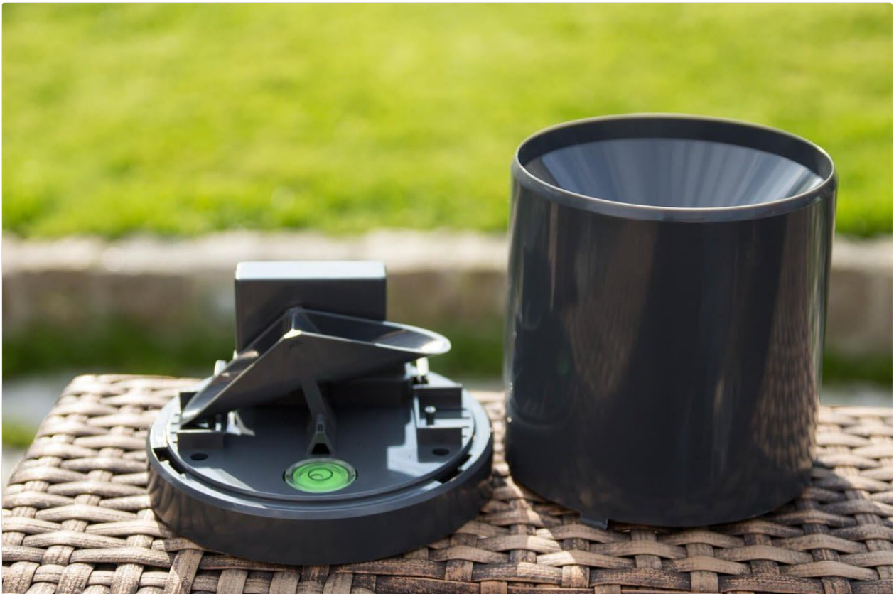
Image: The internal tipping bucket mechanism responsible for measuring rainfall.
