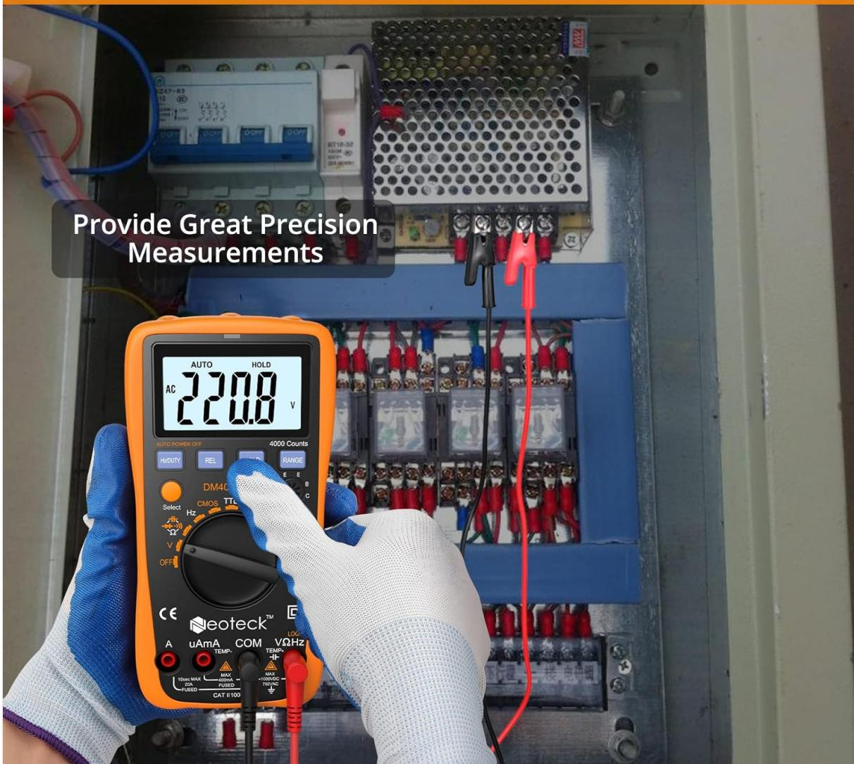
The image shows the Neoteck Multimeter in use, measuring voltage within an electrical control panel. The display shows 'AC 220.8'. The user is wearing gloves, and the multimeter is connected via 15A banana plug to alligator clip cables, providing hands-free measurement.
