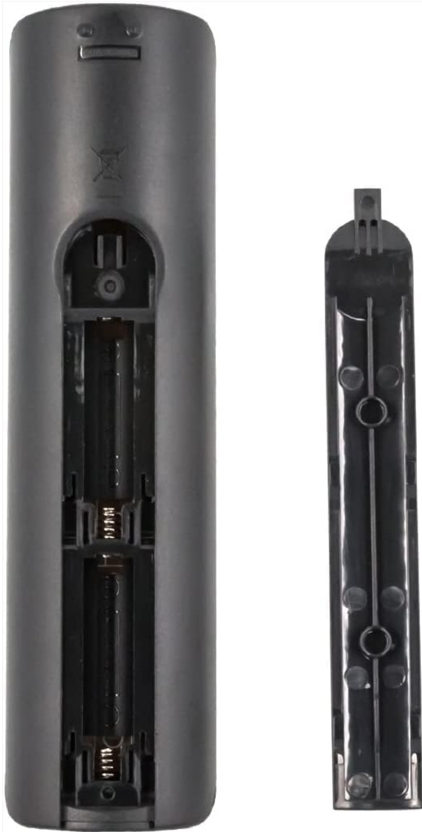
Figure 2: Back view of the remote control with the battery compartment open. This image illustrates where to insert the two AAA batteries.
