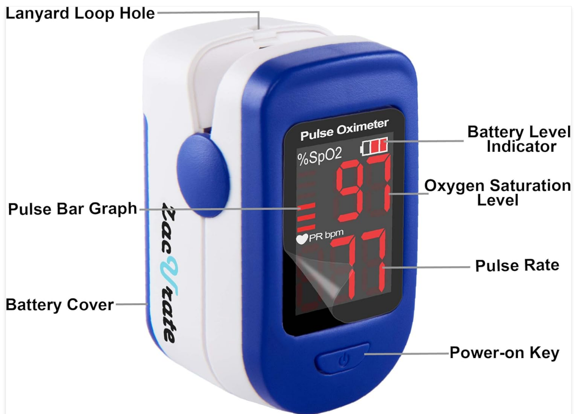
Image: Labeled diagram of the Zacurate 500BL Pulse Oximeter, indicating the power-on key and other components.
