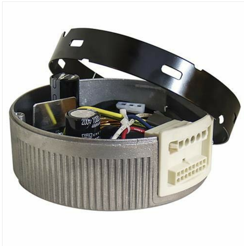
Figure 3: Angled view of the Trane TUY100R9V4W2 ECM Motor Module, showing the top cover slightly ajar, revealing more of the internal circuitry.
