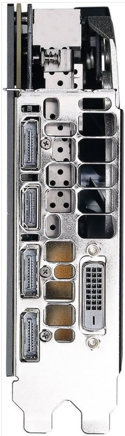
Figure 2: Rear view of the graphics card, highlighting the HDMI, DisplayPort, and DVI output interfaces.
