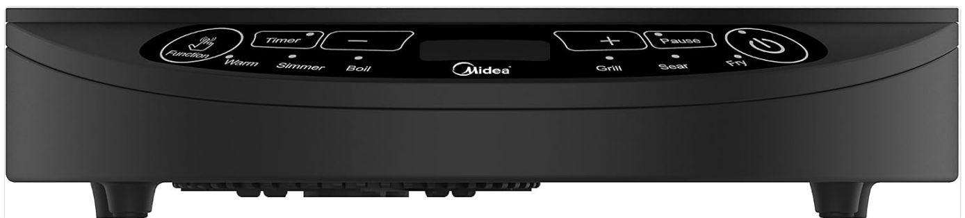
Figure 4.3: Detailed view of the feather touch control panel, featuring buttons for Function, Timer, Power adjustment (+/-), Pause, Power On/Off, and specific cooking modes like Warm, Simmer, Boil, Grill, Sear, and Fry.
