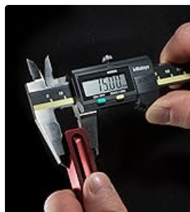
Image: Digital caliper measuring the external dimension of a component.
