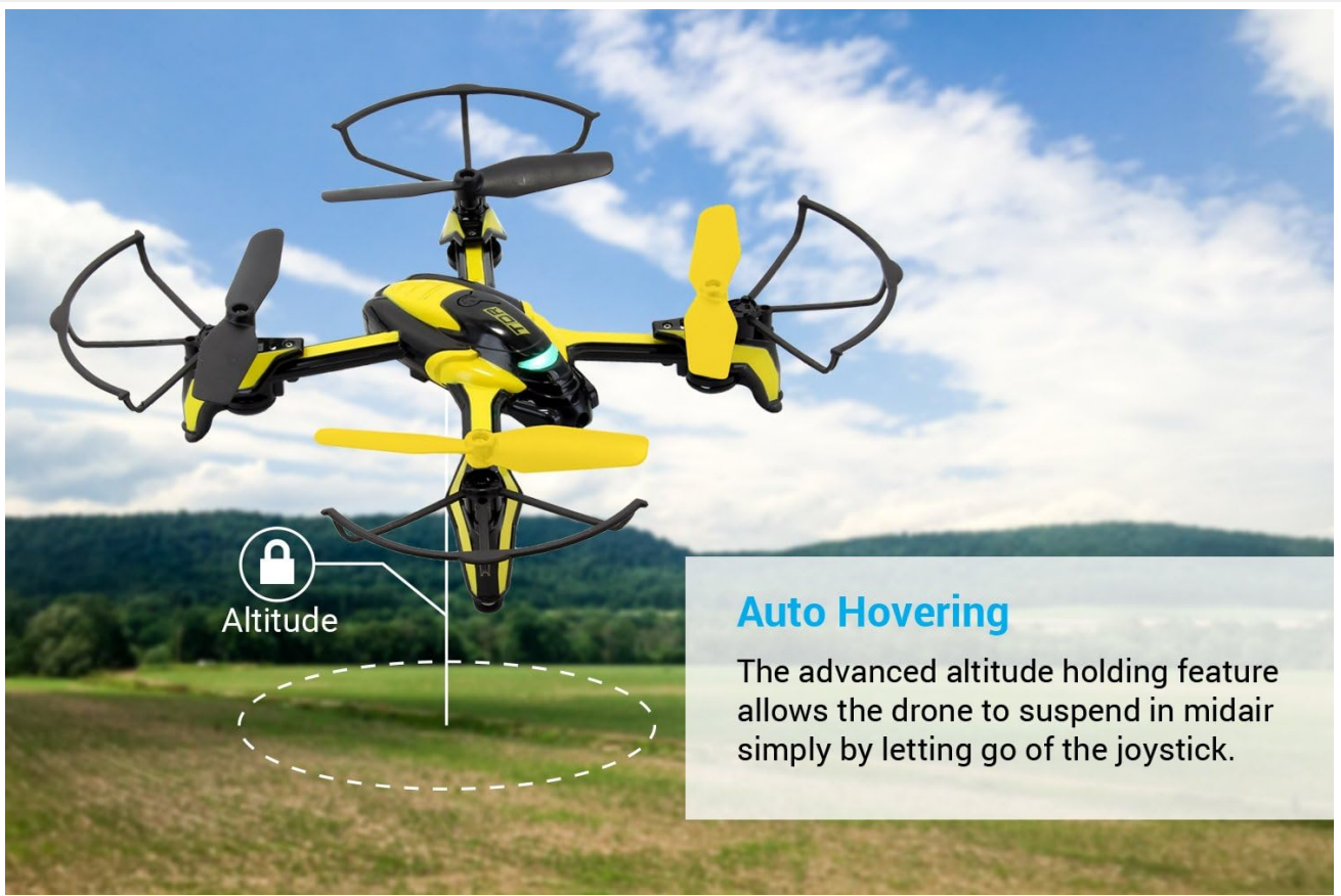
Image: The drone utilizing its auto hovering capability to maintain a steady altitude.
