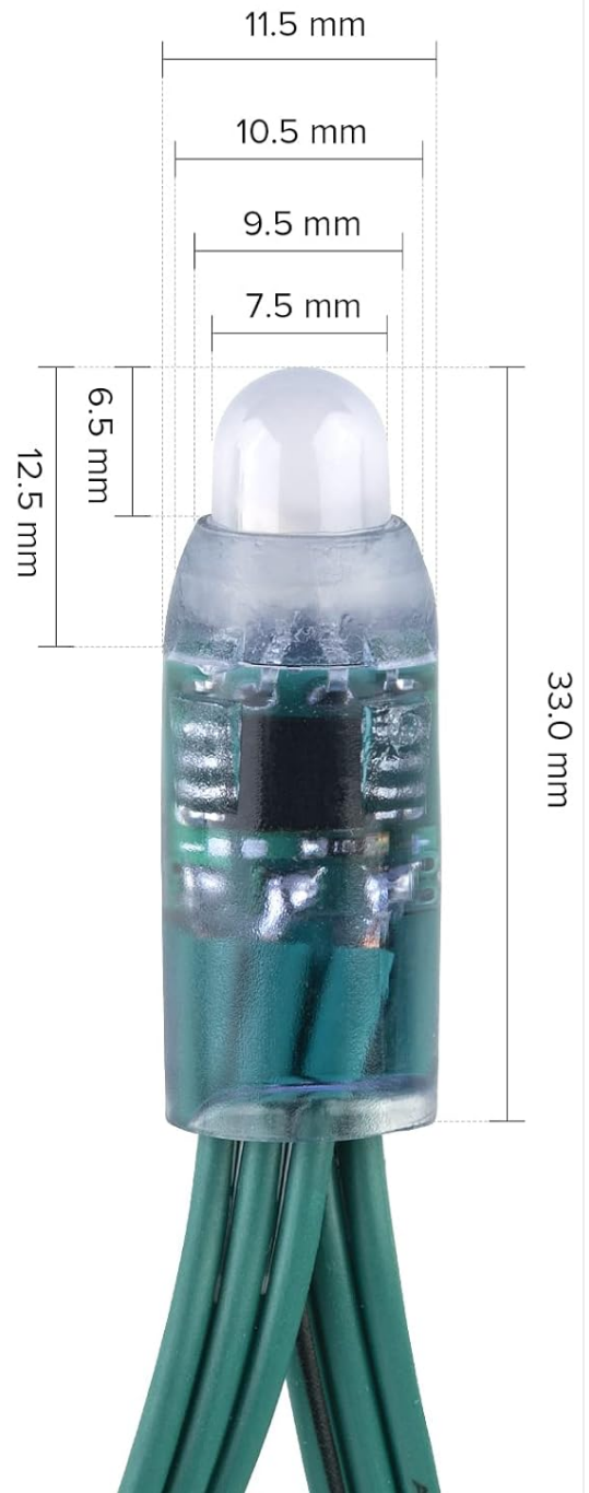
Image 3.2: Close-up of the Smart WS2811 IC embedded within the LED pixel, highlighting its compact design.
