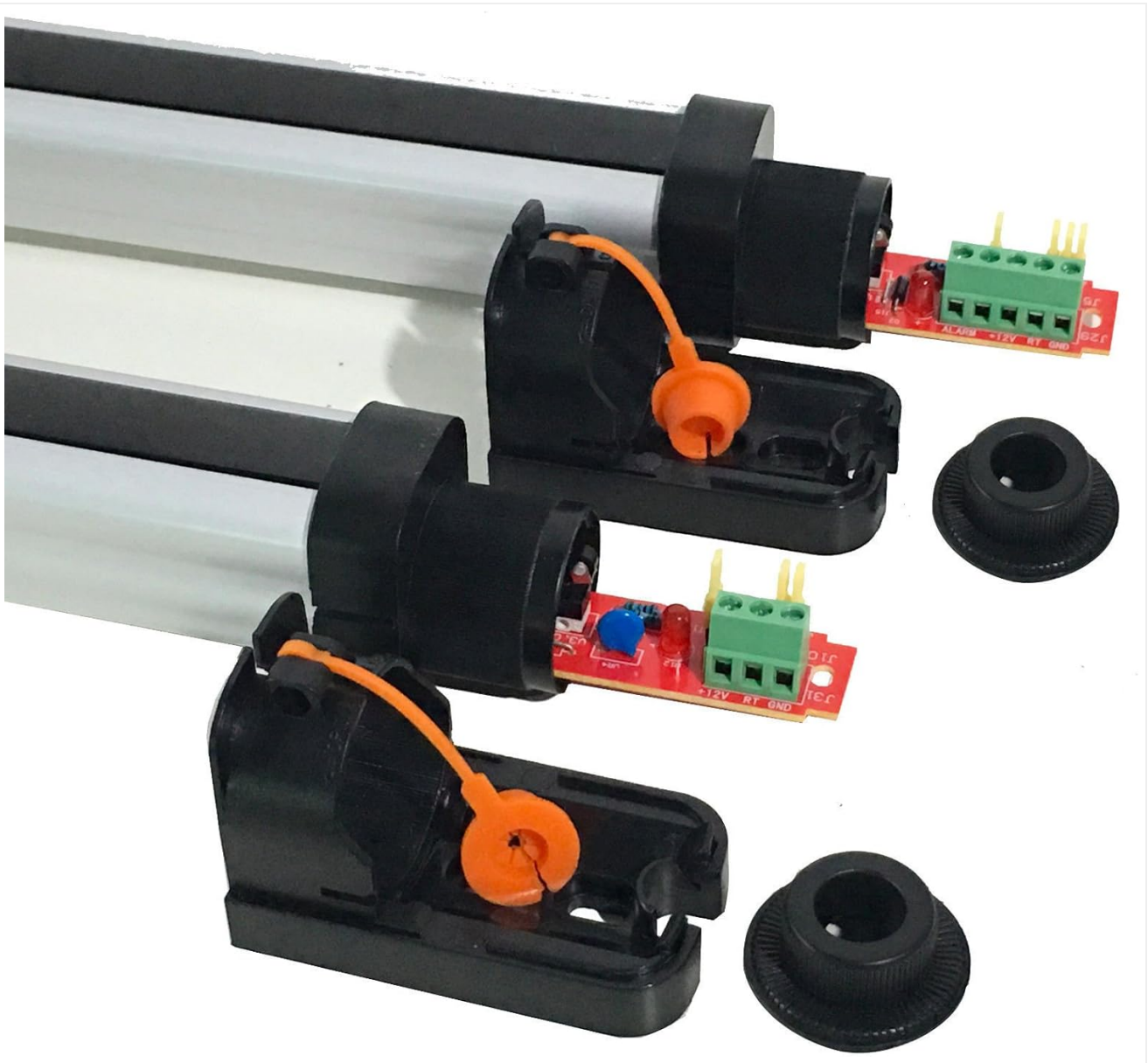
Figure 5.1: Units with covers open, showing circuit boards and wiring access.
