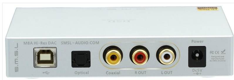
Image: Rear view of the S.M.S.L M8A DAC, showing all input and output ports.
