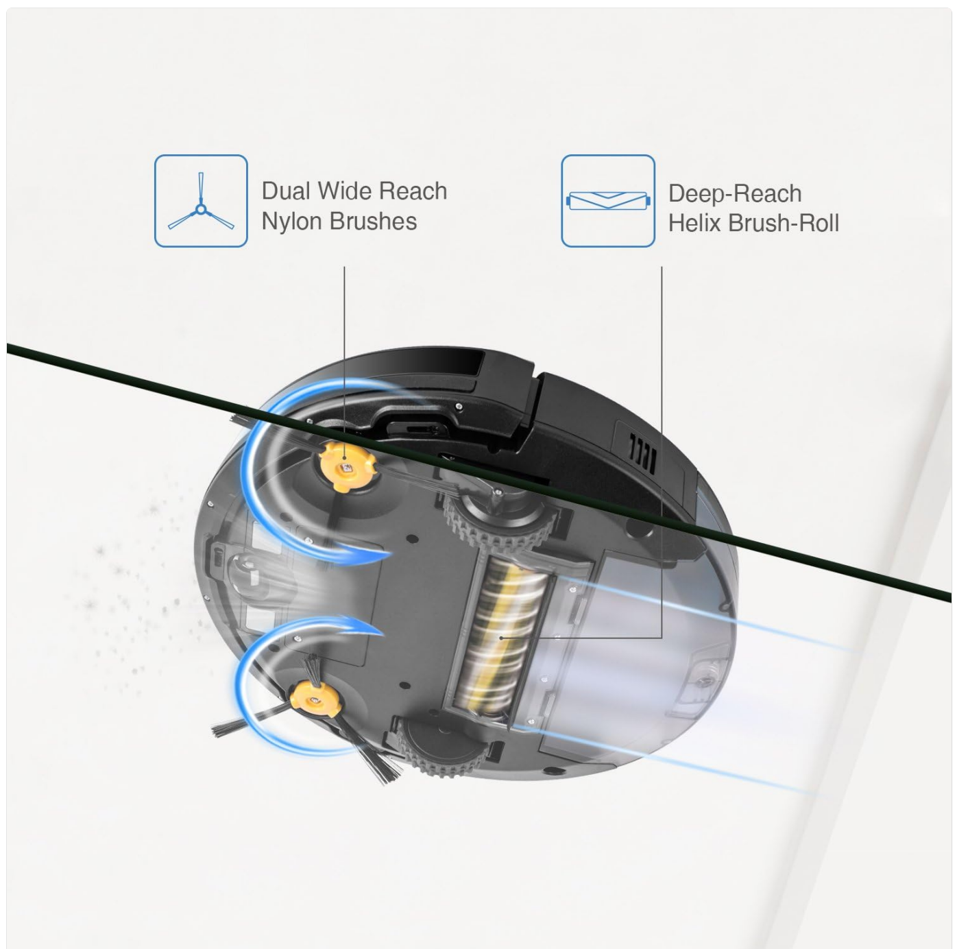
Image: An illustration of the underside of the ECOVACS DEEBOT N79, highlighting the Dual Wide Reach Nylon Brushes and the Deep-Reach Helix Brush-Roll, which are key components for cleaning.
