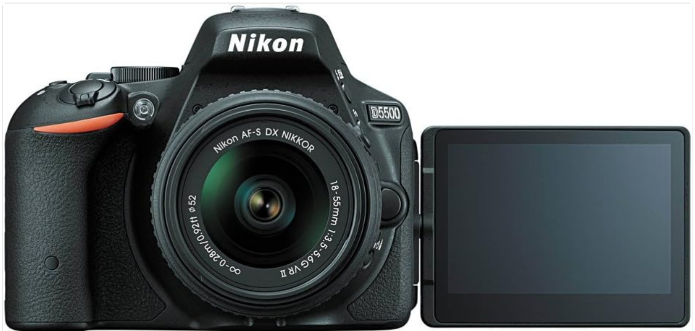
Figure 5: The Nikon D5500 with its vari-angle LCD screen extended, demonstrating its flexibility for different shooting perspectives.
