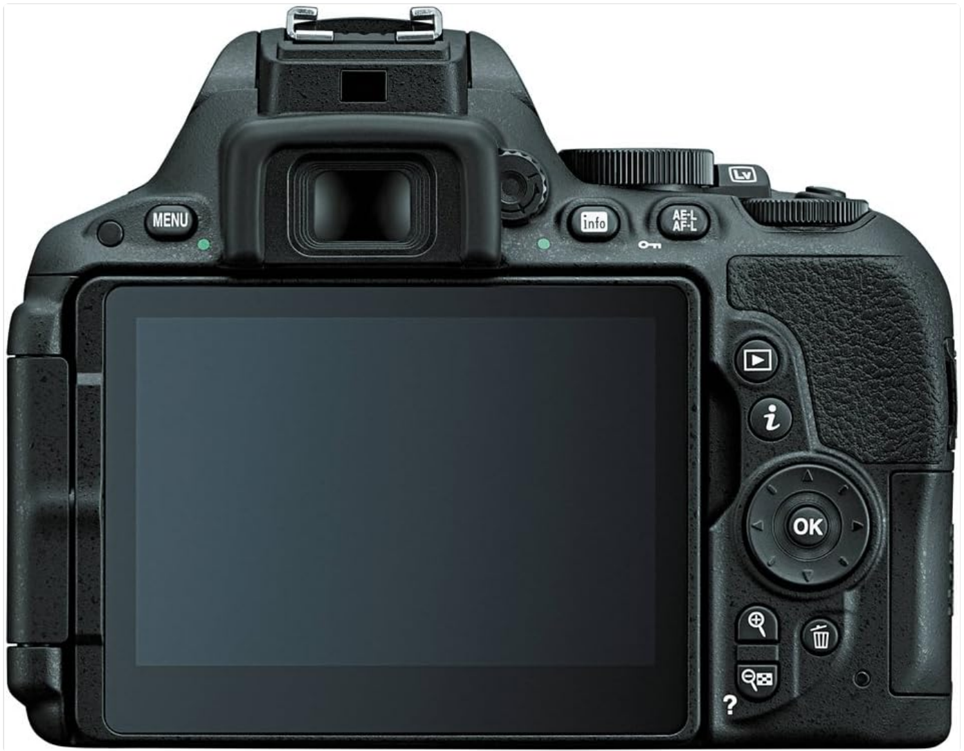
Figure 4: Rear view of the Nikon D5500, displaying the LCD screen and various control buttons for navigation and settings adjustment.
