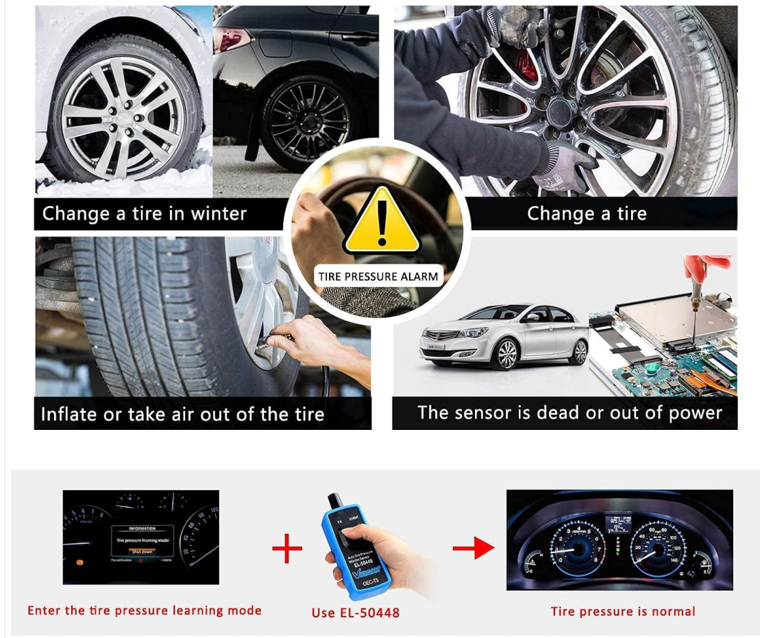
Image 5.1: Common scenarios requiring TPMS relearn, such as tire changes, inflation adjustments, or sensor issues.
