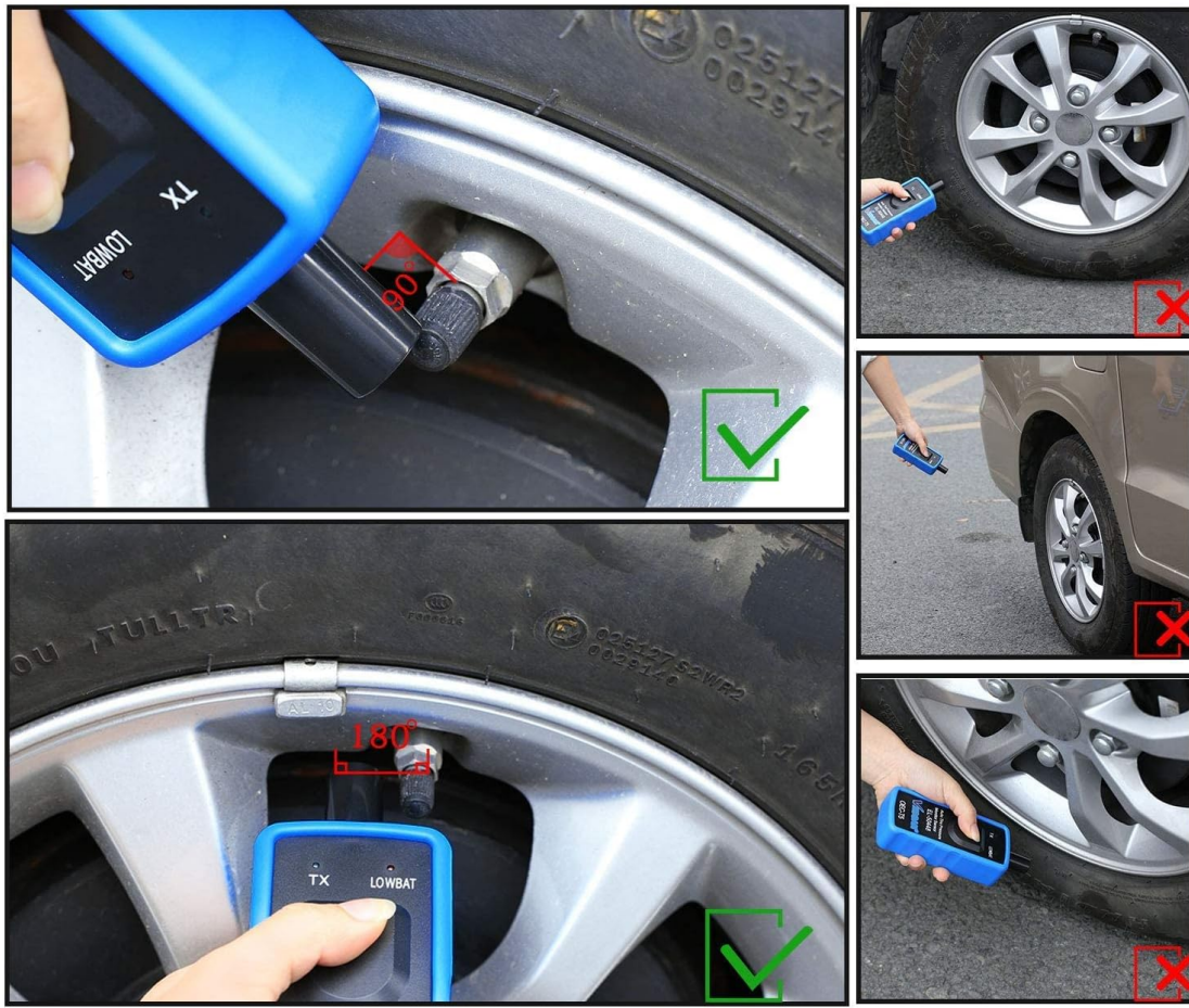
Image 5.3: Illustrations demonstrating correct (90° or 180° close to the valve) and incorrect positioning of the TPMS relearn tool for sensor activation.
