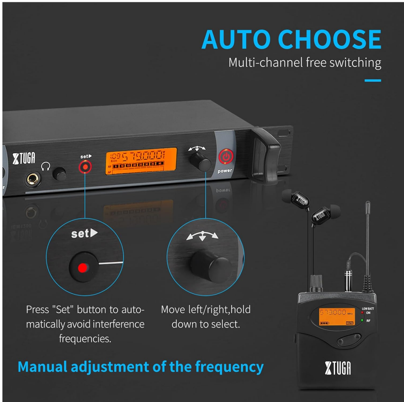
Figure 6: Illustration of the frequency selection process, demonstrating both the automatic "SET" button function and manual adjustment using the left/right controls.
