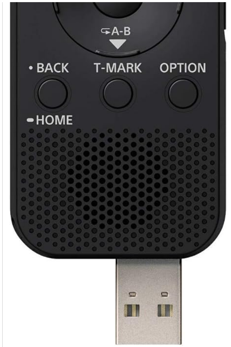
Figure 3: Front view of the recorder with its integrated USB connector extended from the bottom, ready for direct connection to a computer.
