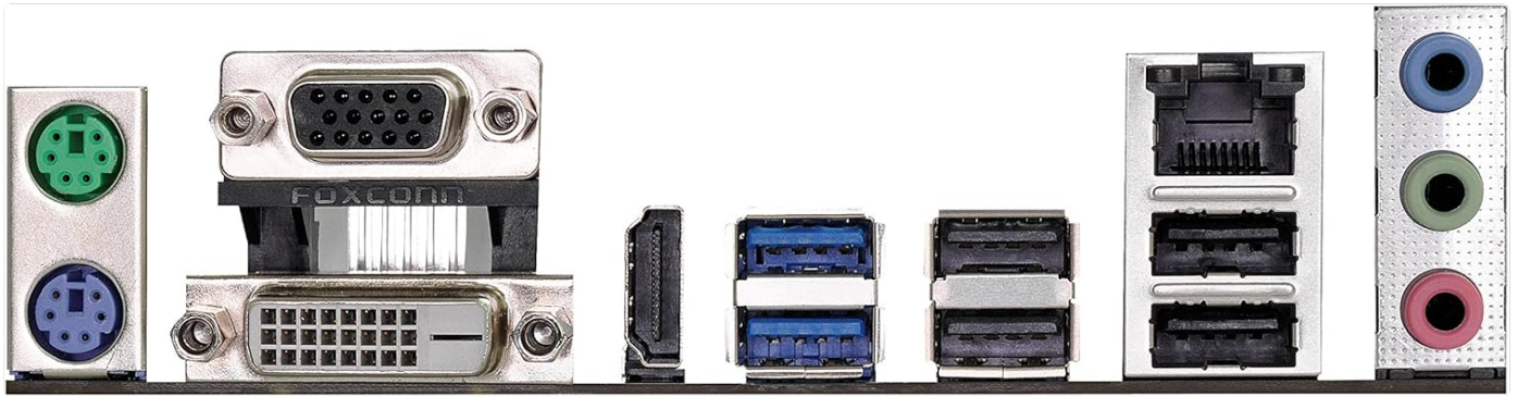
Figure 3: Close-up view of the rear I/O panel, showing PS/2, D-Sub, DVI-D, HDMI, USB 2.0, USB 3.1 Gen1, LAN, and audio ports.
