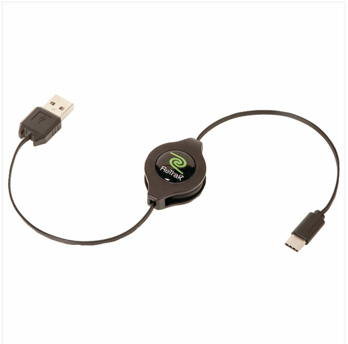
Figure 2: The ReTrak Retractable USB-C Cable fully extended, illustrating the USB-A connector on one end and the reversible USB-C connector on the other, connected by the retractable housing.
