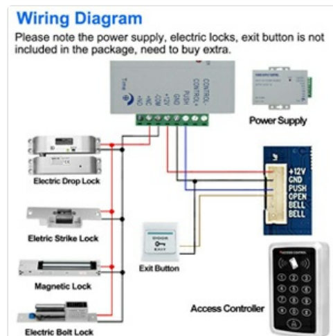
Figure 4.2: Wiring Diagram. This diagram illustrates how to connect the access control keypad to a power supply, various types of electric locks (Electric Drop Lock, Cathode Locks, Magnetic Lock, Electric Mortise Lock), and an exit button.
