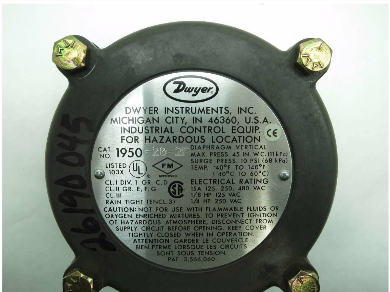
Figure 3.3: Detailed view of the product label, clearly showing the manufacturer (Dwyer Instruments, Inc.), model number (1950-20-2F), electrical ratings (15A 125, 250, 480 VAC), and critical safety warnings regarding hazardous atmospheres.
