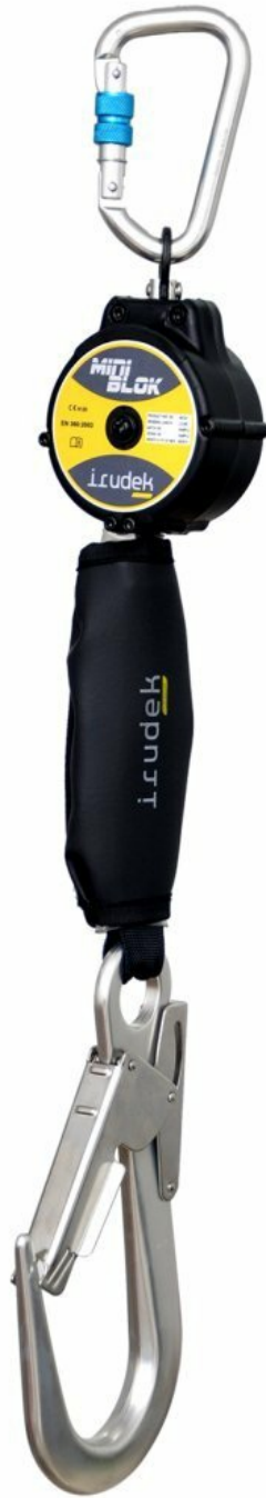
Figure 1: Irudek Miniblok SE-H Retractable Fall Arrester. This image shows the complete fall arrester unit, including the main retractable body, the aluminum screw-gate upper carabiner, the energy absorber sleeve, and the large lower carabiner with a 60mm opening.
