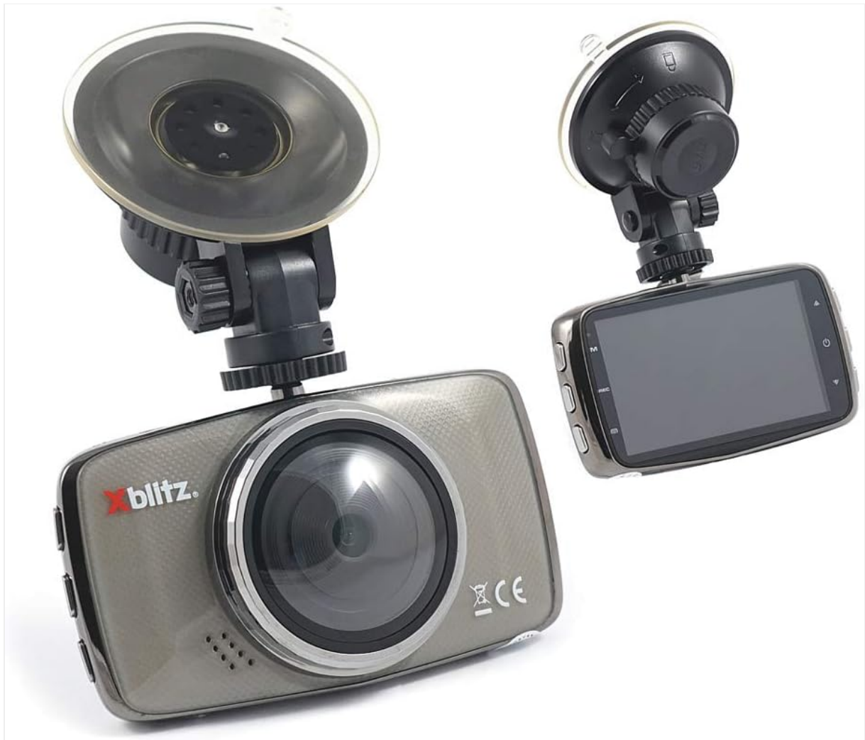
Figure 3.1: Front view of the Xblitz Dual Core main camera with its suction cup mount attached. This image shows the primary lens, the Xblitz logo, and the adjustable suction cup for windshield mounting.
