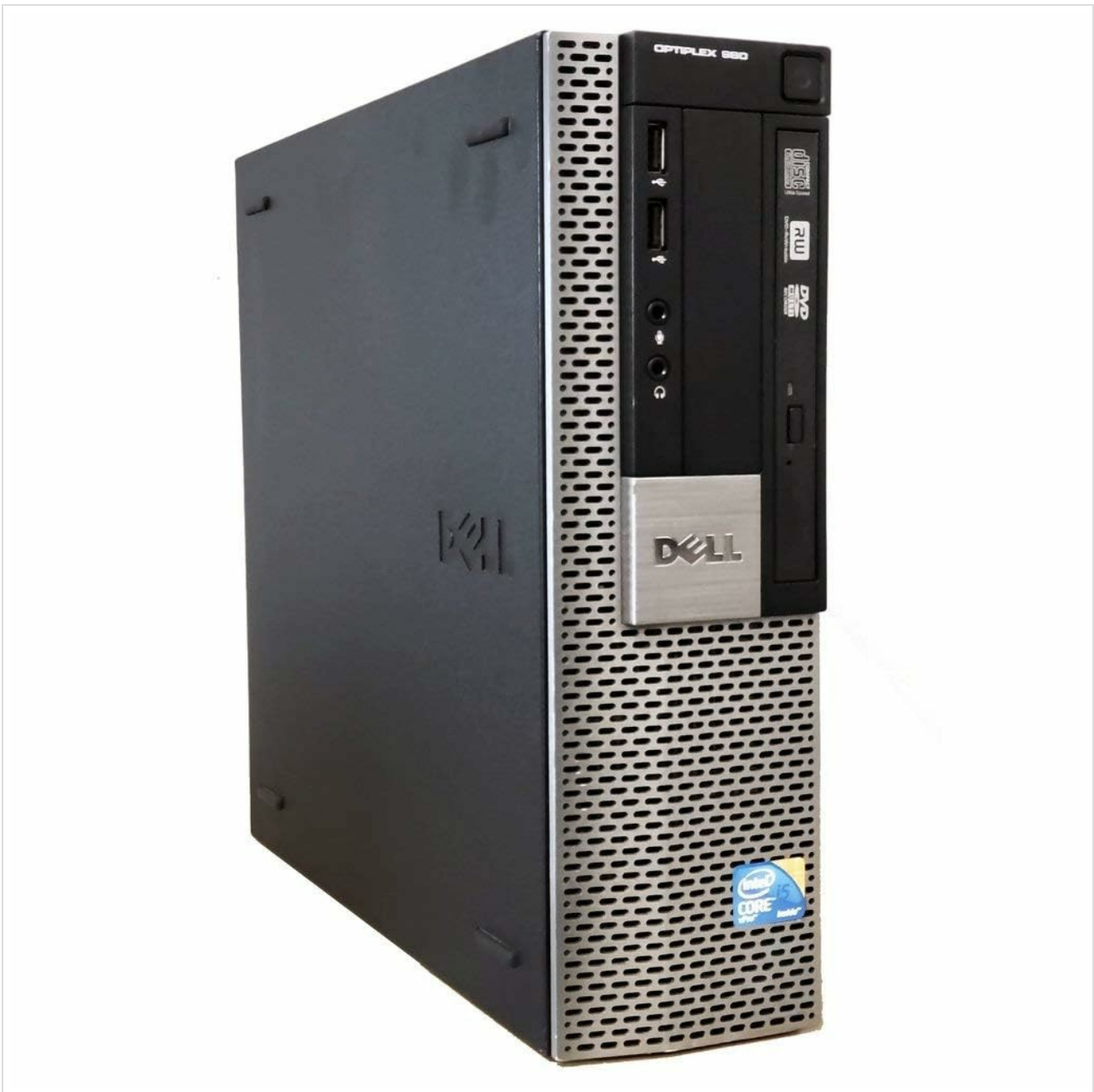
Image: Front view of the Dell Optiplex 980 Desktop PC tower, showing the power button, DVD drive, USB ports, and audio jacks.
