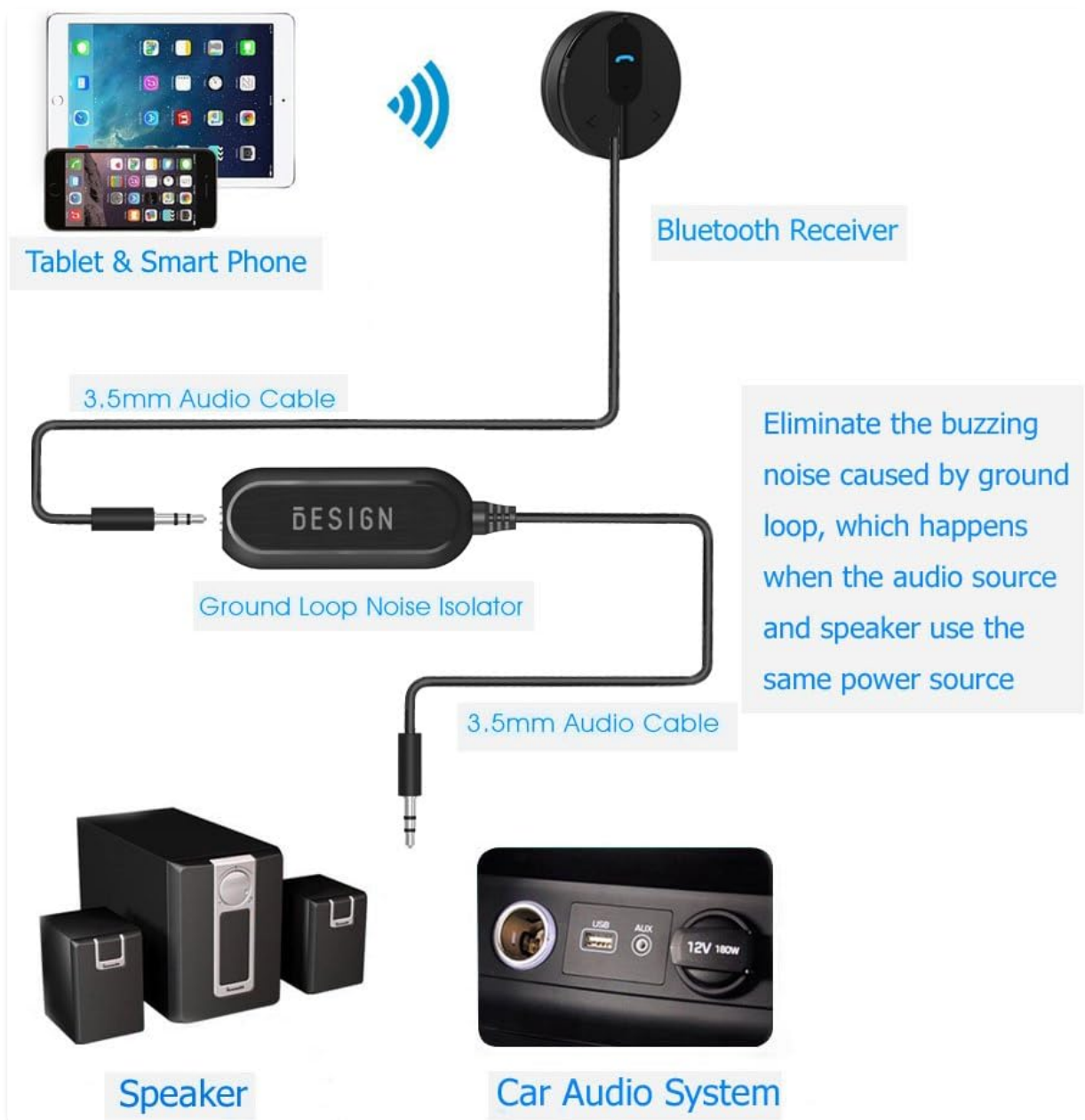
Image: A diagram illustrating how to connect the ground loop noise isolator. An audio source (tablet/smartphone) connects via a 3.5mm cable to the isolator, which then connects to a speaker or car audio system.
