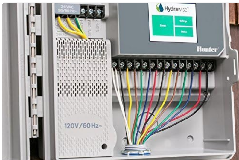
Figure 2: Internal view of the Hunter PRO-HC controller, illustrating the wiring terminal block for zone connections and power input. Connect the 24VAC power supply to the designated terminals. Wire your irrigation zone valves to the corresponding numbered terminals (1-6 for the 6-station model). Connect the common wire from your valves to the 'Common' terminal. If using a master valve or pump start relay, connect it to the 'MV/P' terminal. Ensure all connections are secure and properly insulated.
