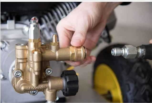
Connecting the high-pressure hose to the pump.
