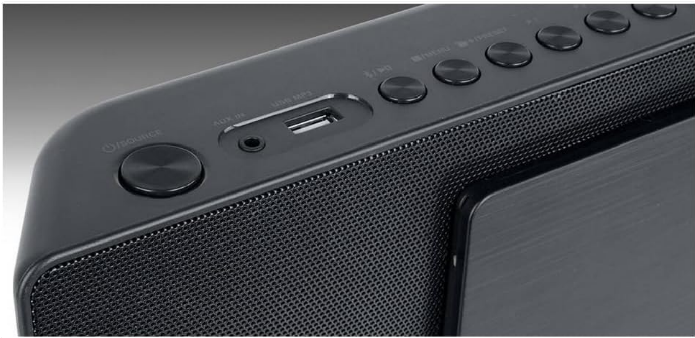
Figure 4.3: Top panel showing various control buttons, the USB MP3 port, and the AUX IN jack.
