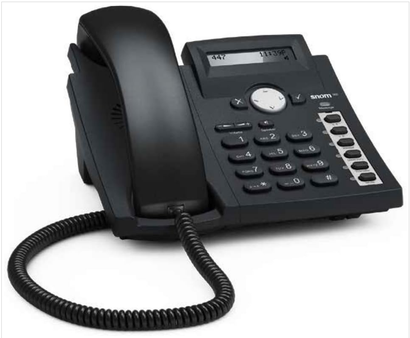
Image 4.1: Front view of the Snom 300 IP Phone, showing the display, navigation keys, dial pad, and programmable function keys.
