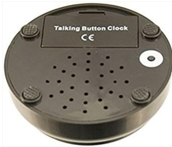
Figure 4: Bottom view of the clock, showing the battery compartment and speaker.
