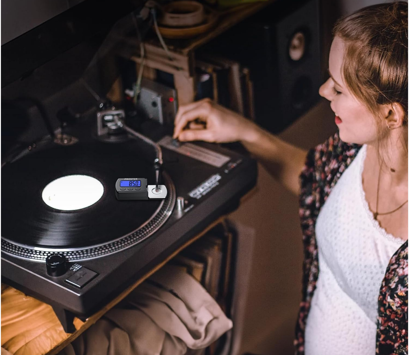
Figure 3.3: Proper placement of the stylus on the weighing platform for accurate measurement.
