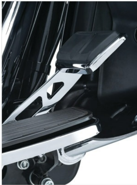
Image 5.1: Close-up view of an installed Kuryakyn extended brake pedal, showing its position relative to the footboard.
