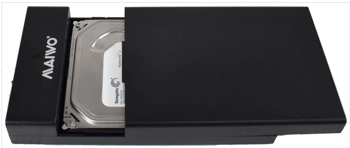
Image: A top-down view showing a 3.5-inch hard drive partially inserted into the Maiwo K3568A enclosure, illustrating the alignment process.
