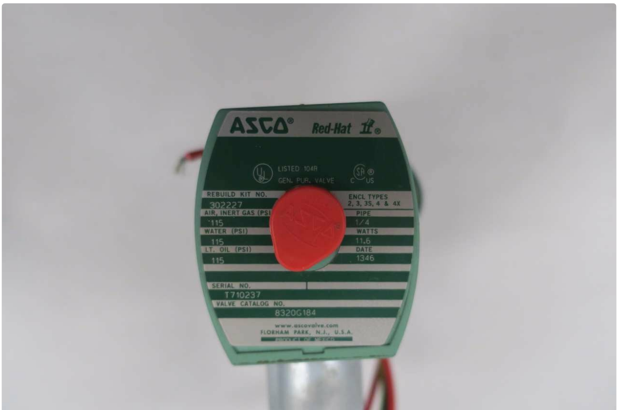
Figure 4: Detailed view of the solenoid coil label, displaying electrical and pressure ratings.
