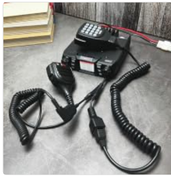
Image: The RJ45 to K1 audio adapter, which allows the BTECH UV-50X2 to connect with a wide range of K1-type audio accessories, enhancing its versatility.
