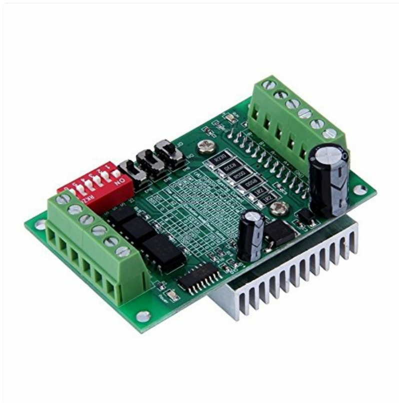
Figure 2: Angled view of the TB6560 board, showing the heatsink attached to the TB6560 chip, which is crucial for heat dissipation during operation.
