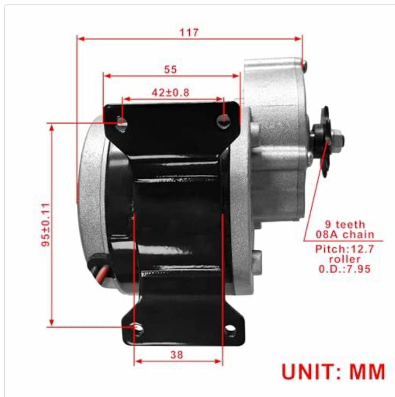
Figure 2: Side view of the motor, highlighting the gear reduction housing and the 9-tooth sprocket on the output shaft.
