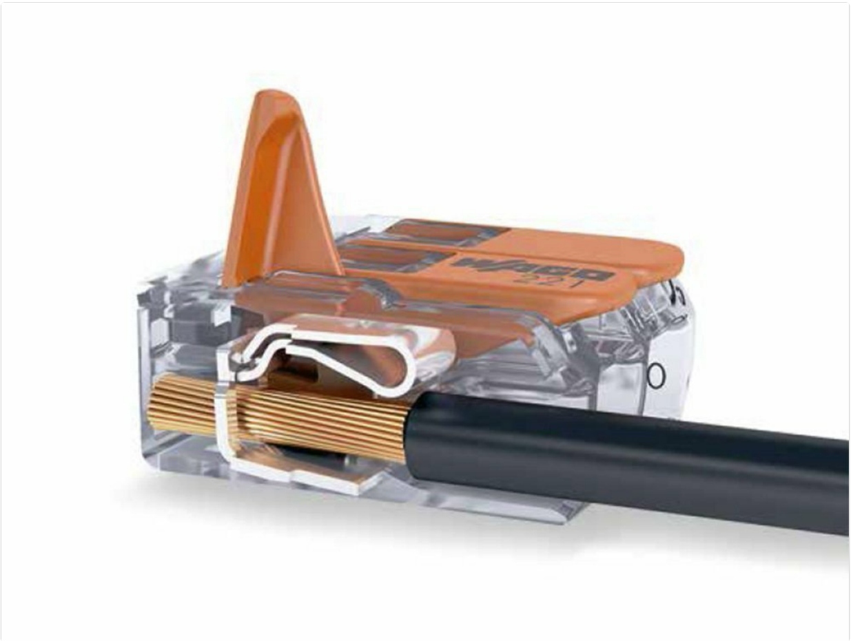
Figure 3: Close-up view of a WAGO 221-415 connector with a wire. A stripped copper wire is shown securely inserted into the transparent connector, with the orange lever in the closed position, indicating a proper connection.
