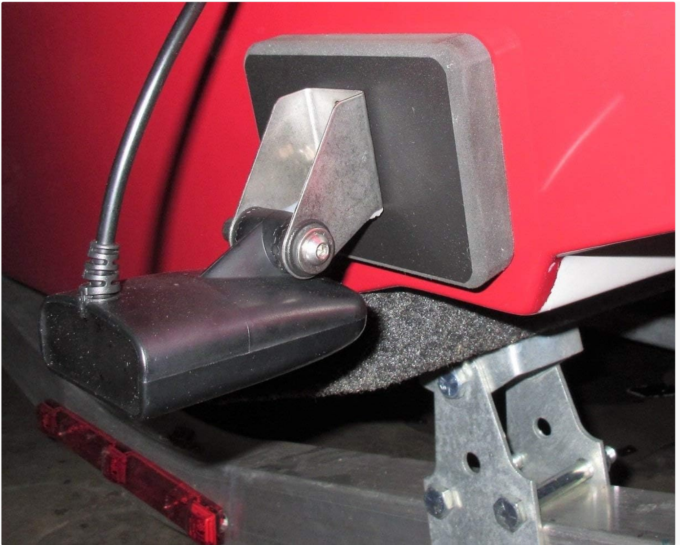
Image: The Stern Pad installed on a boat hull, providing a stable mounting point for a transducer.
