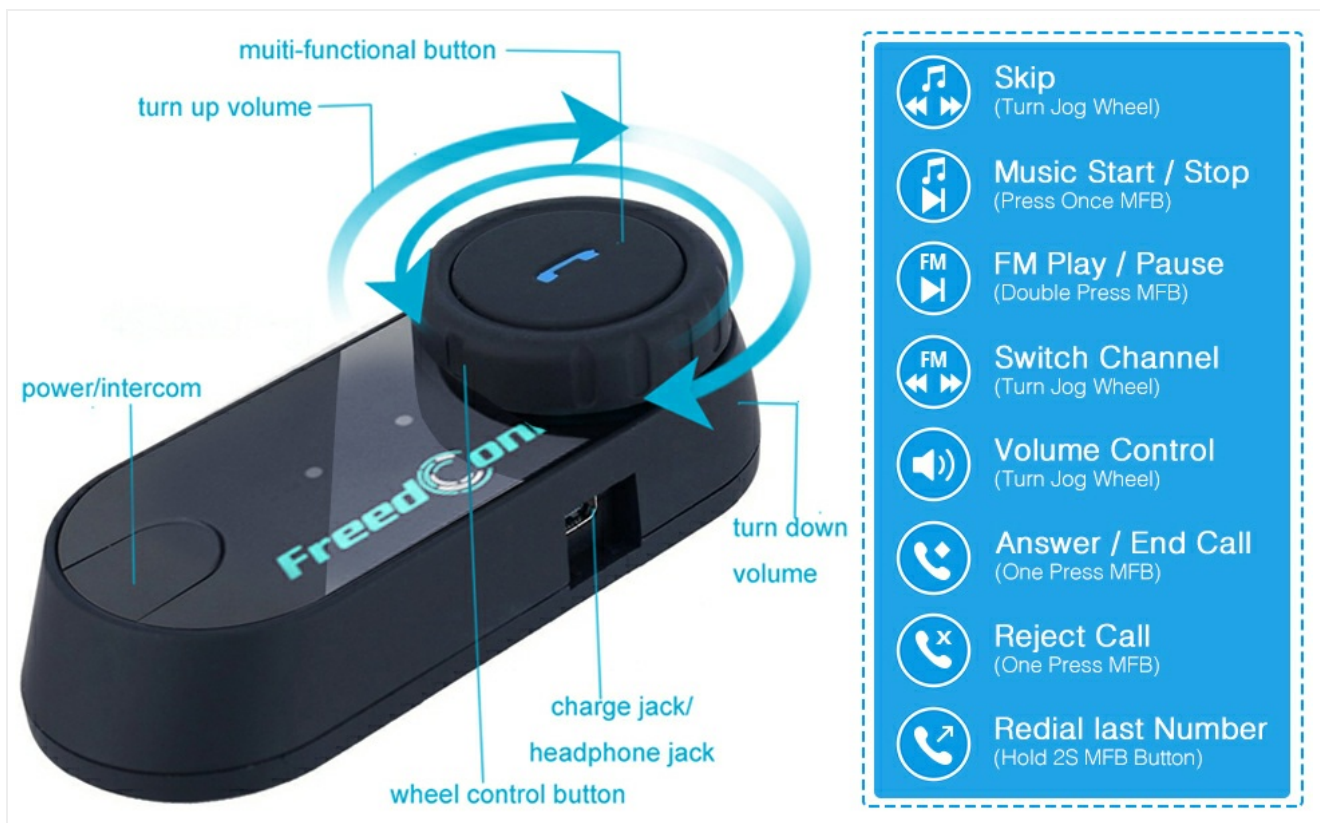
Image: Diagram illustrating the control buttons and ports on the FreedConn TCOM-VB intercom unit.
