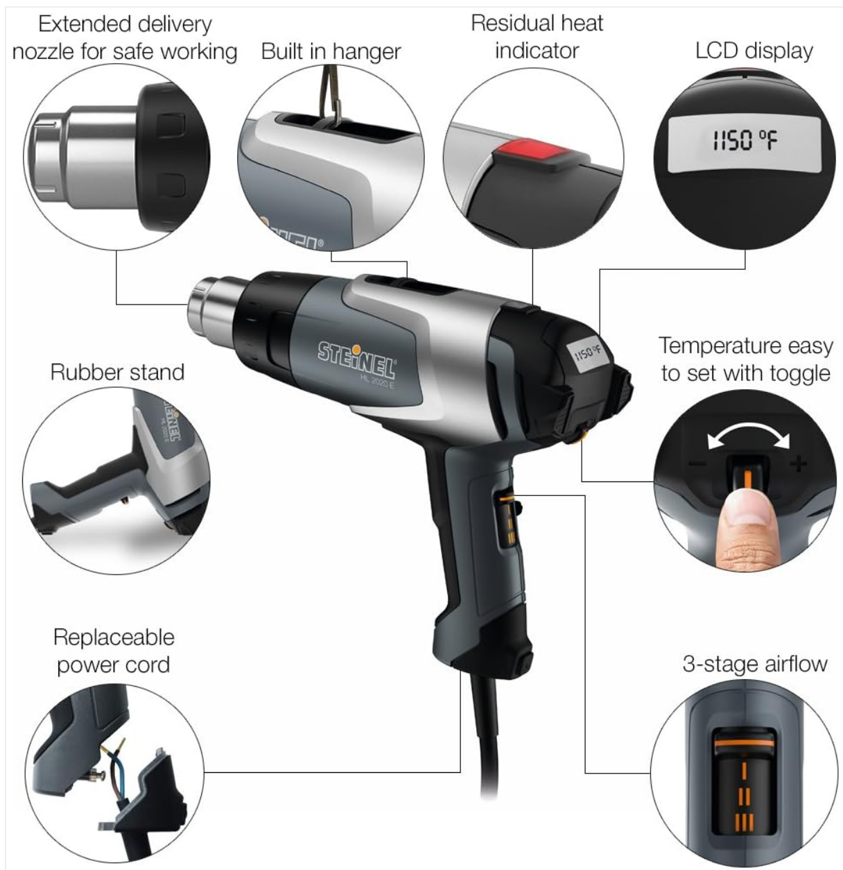
Figure 4.1: Key features of the HL 2020 E Heat Gun.
